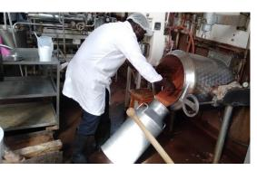
Commercial pasteurizer pulper and harvesting of pasteurized pulp
