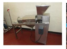
Pulpers are fitted with sieves to separate the seeds and peels from crushed fruit
